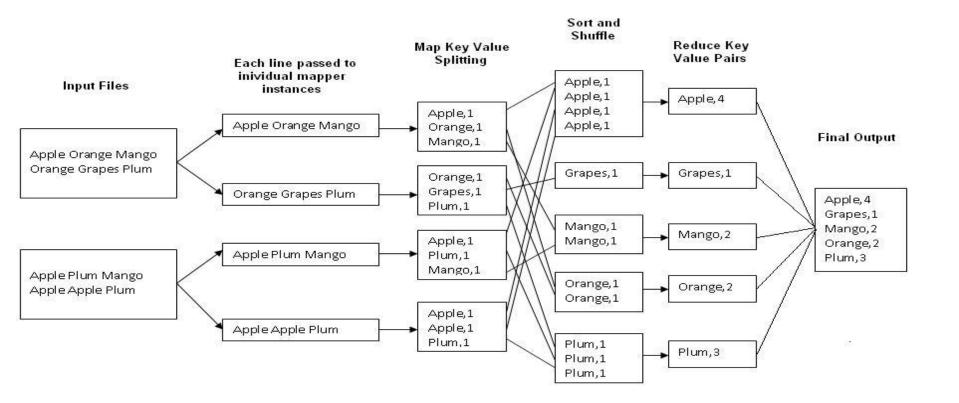
Key/value Pairs: (fileoffset,line)  $\rightarrow$  Map  $\rightarrow$  (word,1)  $\rightarrow$  Reduce  $\rightarrow$  (word,n) file offset is position within the file.
